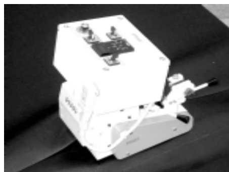
Hot wedge splicing.
